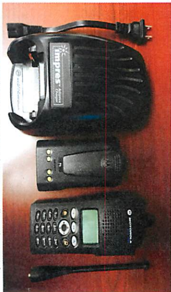
XTS MODEL II, KIT (Charger with AC cord, Battery, Radio, and Antenna).
